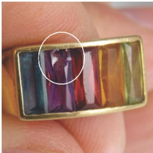
Fig 2.9.1.7 Stone has got damaged due to rough use of setting tools
