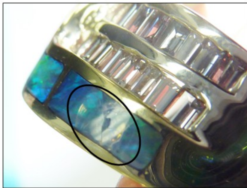
Fig 2.9.1.8 Soft stone has got cracked and damaged due to rough use of setting tools
