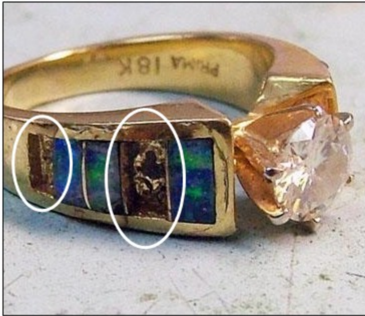
Fig 2.9.1.9 Soft stone has got completely damaged due to rough use of setting tools
